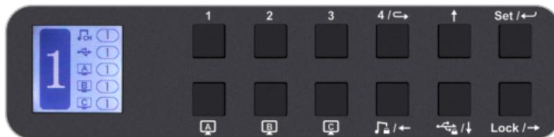
When you use the front panel button or IR remote to control the KVM, the LCD display will inquire your target action, then execute the command according to your operation. The LCD interface in the figure above is the main interface.
