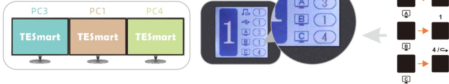
In this mode, each input and output port on the KVM is marked with a letter, and the screen corresponding to the output port is output by the port with the corresponding letter of the PC selected. As shown in the figure above, the screen output by the monitor connected to Output A is from Input A of PC 3, the screen on Output B is from Input B of PC 1, and the screen on Output C is from Input C of PC 4.
