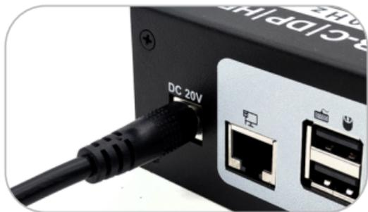
10. By now, the connection has been completed. Turn on the power supply and the KVM Switch will begin to work.
