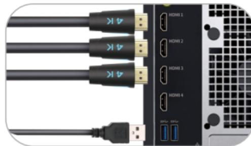
4. Connect external mouse and keyboard to KVM's keyboard and mouse input port.
