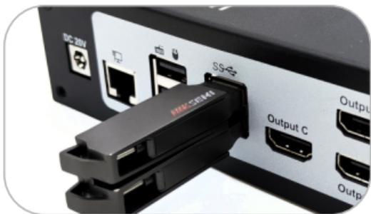
6. Connect KVM's HDMI output ports to 3 HDMI displays with 3 HDMI cables.
