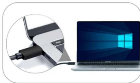
2. Connect PC 2 with 1 DisplayPort cable and 1 USB 3.0 cable. Use DP cable to connect PC 2 to the DP port on the KVM, use USB Type-A end to connect PC 2 and Type-B end to connect the KVM.
