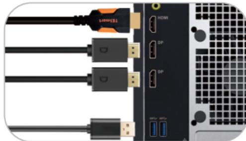
2. Connect KVM's HDMI output ports to 3 HDMI displays with 3 HDMI cables.
