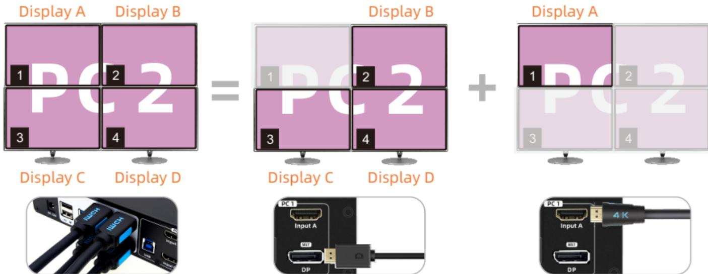
**Tips:** If a device that doesn't support MST is connected, the display will only show on output A or show three duplicated screens. The specific situation depends on the device.
