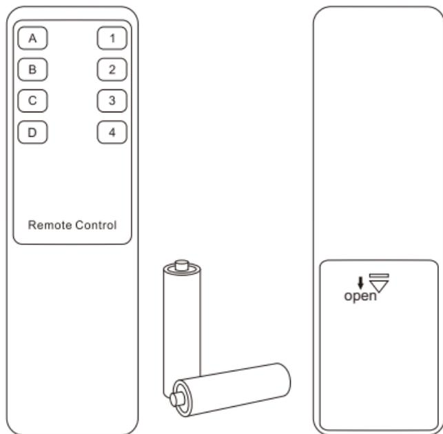
**Tips:** By default, the remote control is not equipped with batteries, due to the safety requirements of some express companies. Install AAA dry cells before use.
