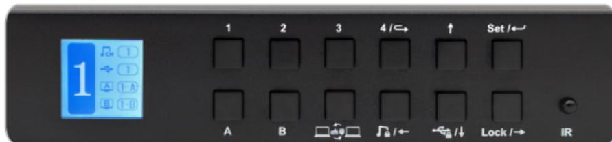
When you use the front panel button or IR remote to control the KVM, the LCD display will inquiry your target action, then execute the command according to your operation. The LCD interface in the figure above is the main interface.
