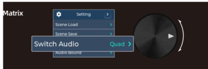
**Tips:** When you switch audio channel on any output, both the L/R audio and the display audio of that output will be switched at the same time.
