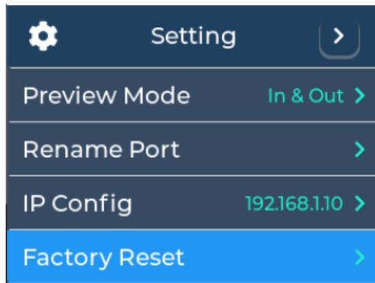
**Tips:** 1. When you want to return to the previous menu level, you can press the “:≡” button to return, or you can rotate the dial to the return button at the top right of the LCD and press to return.
