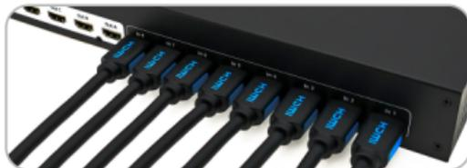
2. Connect 8 display devices to the HDMI output ports above each "Out" logo of the Matrix using 8 HDMI cables.
