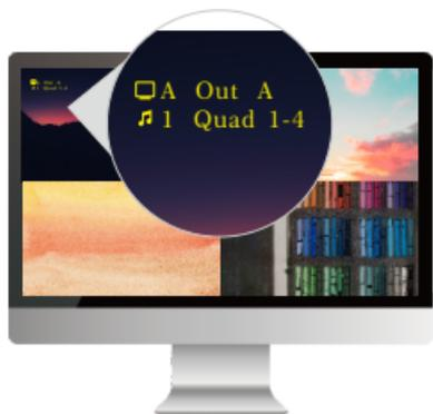
The yellow “🎵” icon in the upper left OSD will also indicate the currently sound channel. The number displayed after the icon is the input port number of the actual output audio.
